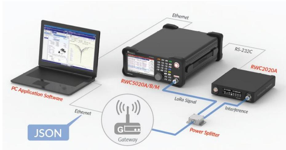
Fig 3.30 Interferer test environment
